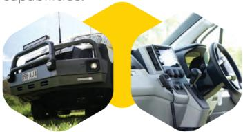
As a 12 seater this vehicle can be driven on a standard drivers licence. It has a 2.8L 4-cylinder turbo diesel engine with automatic transmission. The suspension upgrade includes a 180mm lift and a GVM (Gross Vehicle Mass) increase to 4.3T. With additional mine specs including seat belt alarm, Internal Roll Over Protection System (ROPS), VHF radio and In Vehicle Monitoring System (IVMS) the vehicle can be customised to suit all major mine site requirements including BMA Spec.
